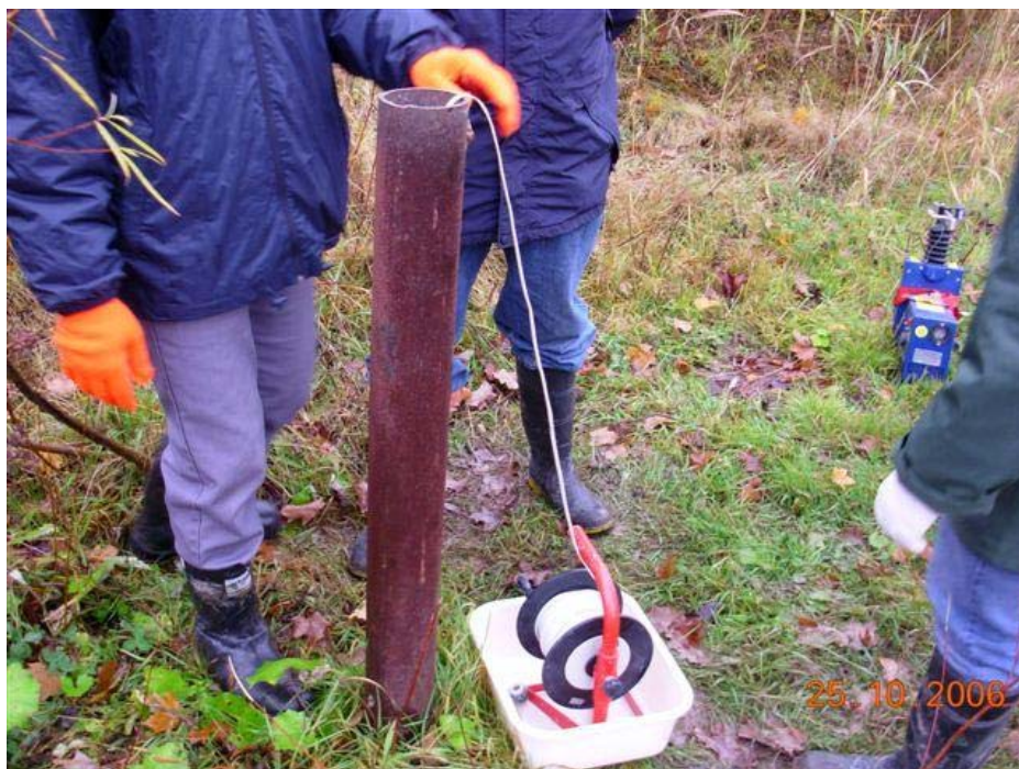
Photo 2. Initial measurement of water level in the observation well (MDDEP, 2006)
