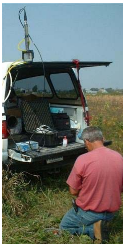
Photo 8. Measurement of physicochemical parameters. The measuring cell is on the roof of the car (MDDEP, 2010)
