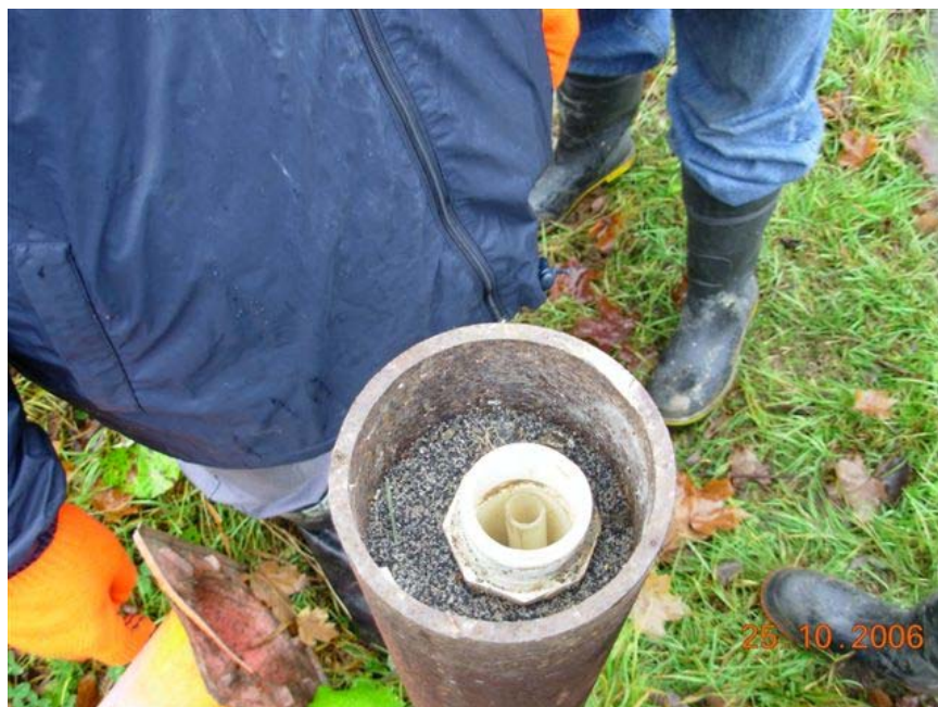
Photo 6. Overhead view showing the protective casing, the PVC inner casing and the tubing in position for the purge. Note that the annular space above the ground has been filled with granular material to support the casings (MDDEP, 2006)
