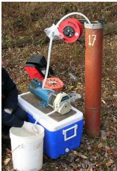
Photo 7. Purge of a predetermined volume from the observation well. Both drawdown (note the piezometric probe) and volume pumped (container blank) are controlled throughout the operation (MDDEP, 2006)
