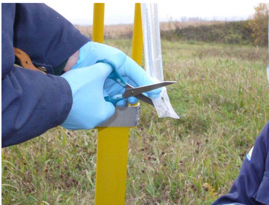
Photo 10. Operation to recover the sample in a diffusion bag: gloves and scissors must be free of contaminants (MDDEP, 2008)
